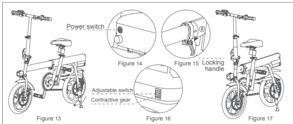
1 Fold the kickstand, lower the head and saddle height to the minimum (see Figure 13). Turn on power (see Figure 14), release the locking handle (see Figure 15 - ⑧ arrow); set right the body, put the adjustable switch in the contractive gear (see Figure 16). The body automatically folds, and when finishes, put the adjustable switch in the stop gear, close the locking handle, turn off the power (see Figure 17).
