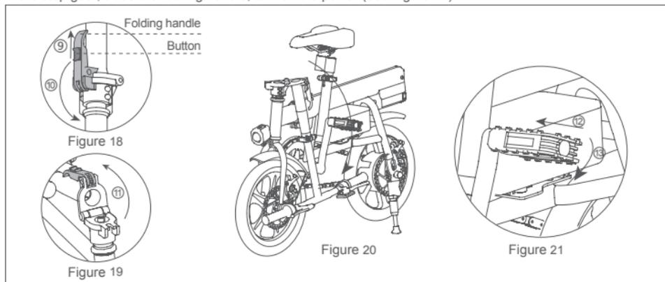
2 Push the button on the folding handle (see Figure 18- ⑨ arrow) and fold down the folding handle (see Figure 18 - ⑩ arrow) to fold the head as shown in Figure 19 - ⑪ (see Figure 20). The pedals are pushed down (see Figure 21- ⑫ , 21 - ⑬ arrow), and fold the pedals to complete the folding.
