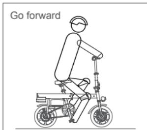
Turn the accelerator handle down with right hand to accelerate
