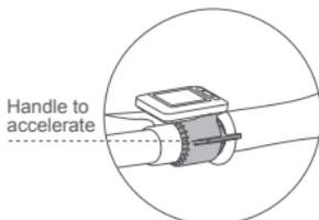
Turn the accelerator handle down with right hand, and the motor speed increases. Release and go back to zero gear.
